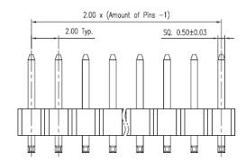
Pins assignment for PCB Layout
