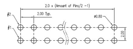
Recommended P.C.B. Layout Layout Tolerance =  $\pm$  0.05 mm
